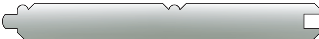
T&G 15 5/8"x 5 1/8" Face CVG Hemlock T & G, #708 Face, Edge & Center Bead Back
